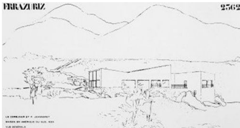
Figure 1: Maison Errazuriz A rendering done by Le Corbusier for Eugina Errazuriz's proposed house design showcasing the first use of the butterfly roof. Unfortunately, it was never built.
