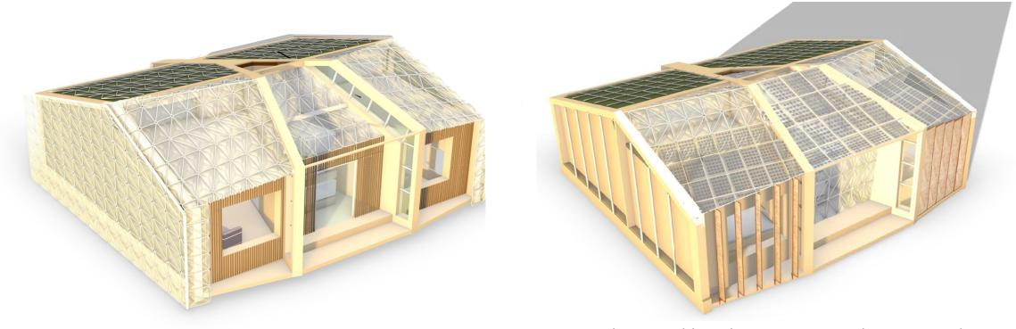
Non-Operable ETFE Membrane to create controlled environment for plant growth
