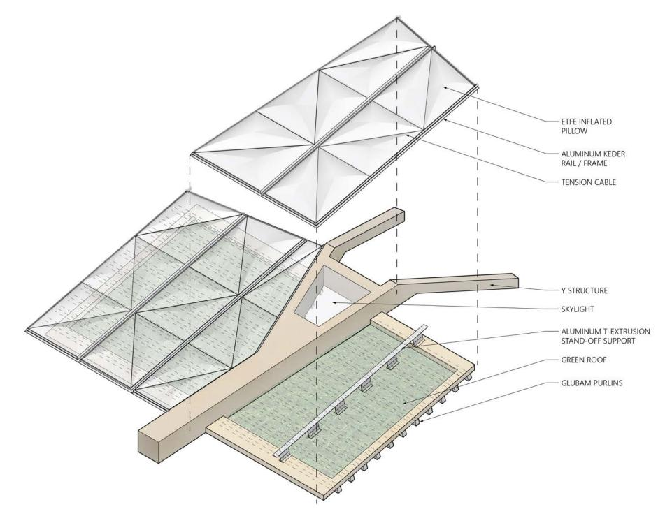
EXPLODED ROOF CONSTRUCTION
