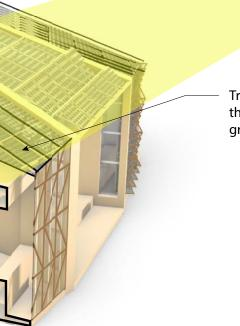
Translucent Solar Panels that use the same structural grid as the ETFE.
